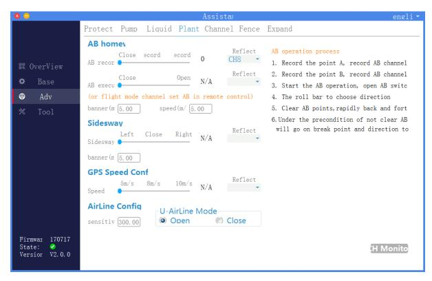
**2. Operation:** the maximum flight speed can be limited at 5m/s,8m/s or 10m/s by switching the control stick when the aircraft is flying under GPS speed mode.
