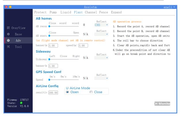
**3. Operation:** switch to "Close"—"Move to the left"—"Close", and it will execute a left side-move once; switch to "Close"—"Move to the right"—"Close", and it will execute a right side-move once.
